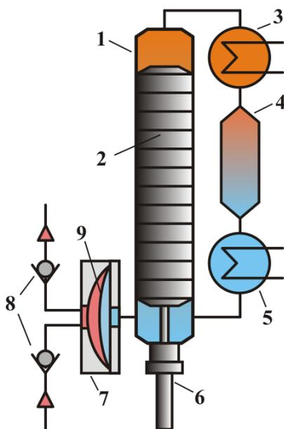
It consists of a cylinder (1), filled with a liquid working fluid, with a piston (2) inside. The piston divides the internal volume of the cylinder into two parts – hot and cold, shown in orange and blue. Both parts are communicated through a heater (3), a regenerator (4) and a cooler (5) connected in series. The reciprocating
